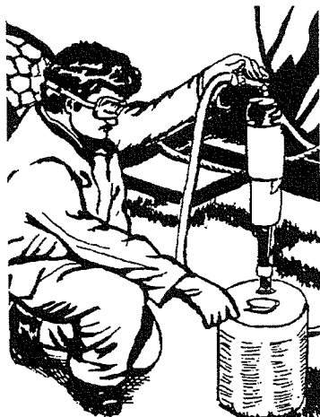
Figure 6-18. The safest way to transfer hazardous pesticides from their containers into mixing tanks is with a closed handling system. Many closed handling systems will rinse the empty containers.
