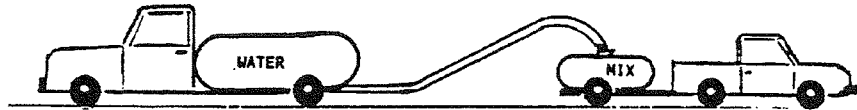
Figure 7-6. A sewer jetter provides a convenient source of water for filling application tanks and eliminates back-siphoning possibilities.
