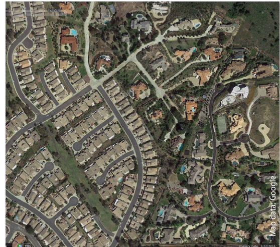
Figure 11. High- versus low-density development north of Poway, California. Tighter clustering of housing decreases amounts of flammable vegetation, which makes defensible space easier to maintain. During a wildfire, high-density development can also be defended more easily and with fewer resources.
