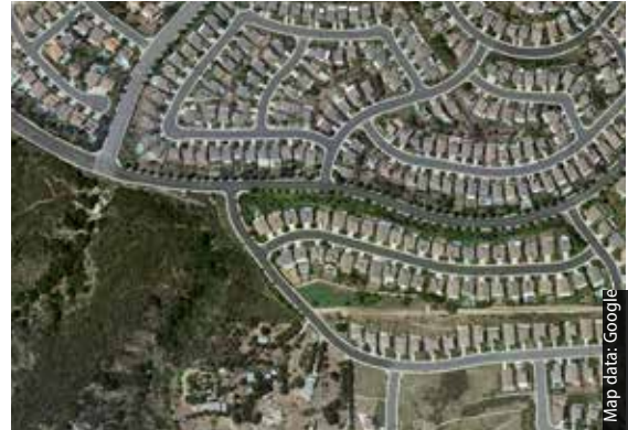
Figure 10. Localized concentration of homes on the inner side of a perimeter road near Alberhill, California. Roads, sidewalks, and yards all become defensible space between the wildlands and structures when homes are sited in this fashion.
