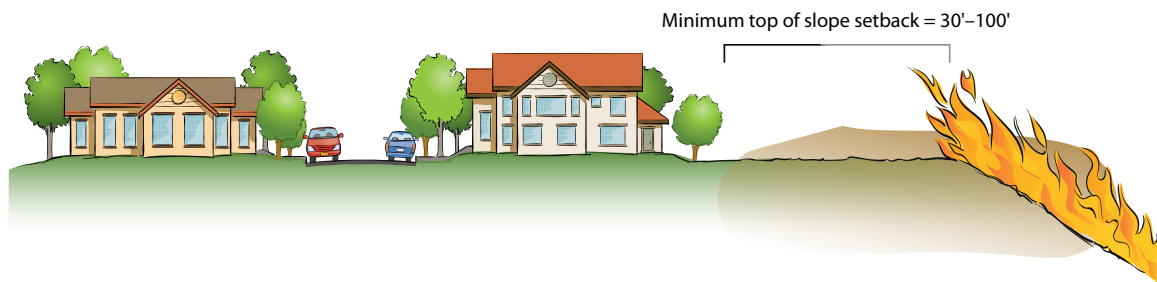
Figure 9. Development near slopes should be set back far enough from the slope's edge to provide safety from flames traveling upslope or lapping over the edge. Most guidance recommends a minimum safety area in the immediate "home ignition zone" of 30 feet; however, depending on the height of buildings and the potential flame lengths of burning vegetation on the slope, up to 100 feet may be needed.
