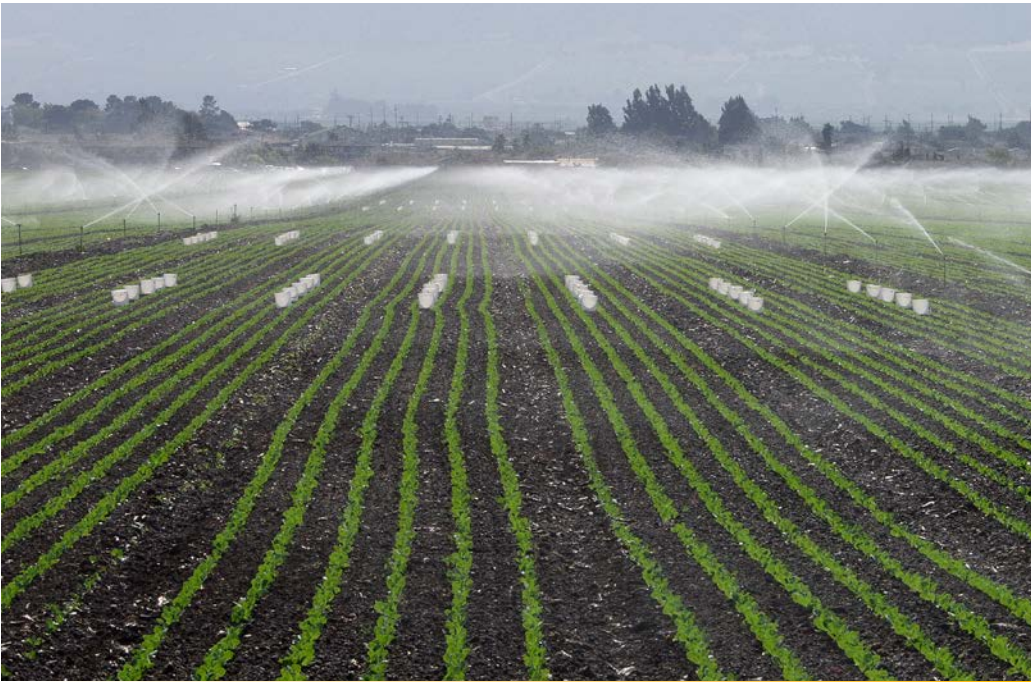
Figure 2. Grids of evenly spaced buckets set up in several locations in a field can be used to determine if a sprinkler system is applying water uniformly. Photo: M. Cahn.
