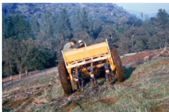
Figure 10. A rangeland drill seeding in an oak woodland following woody plant control.
