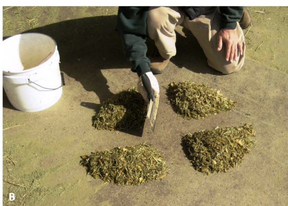
Figure 4. Dumping (A) and quartering (B) sample. The intermediate stage of mixing is not shown.
