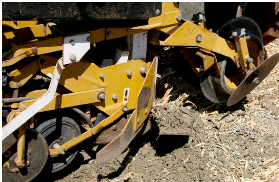
Figure 5. Close-up of Buffalo ridge-tillage planter showing residue-clearing hiller disk (right), sweep (center), and seed shoe and closing wheel (left). Photo: J. P. Mitchell.
