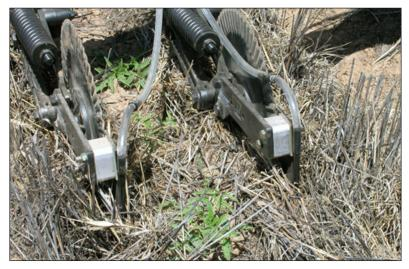
Figure 5. Applying liquid fertilizer as a side-dress to fresh market tomatoes in Parlier, California, conservation tillage study, 2002. *Photo:* J. P. Mitchell.
