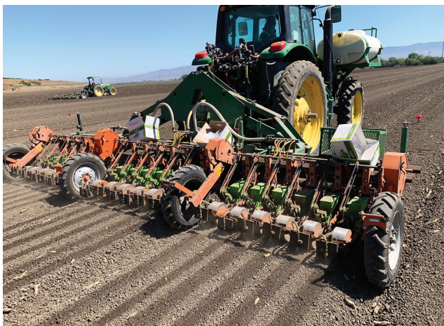
Figure 4. Direct-seeding six seedlines of lettuce on a bed 80 inches wide. Anticrustant and herbicide are applied over the top of the seedline.
