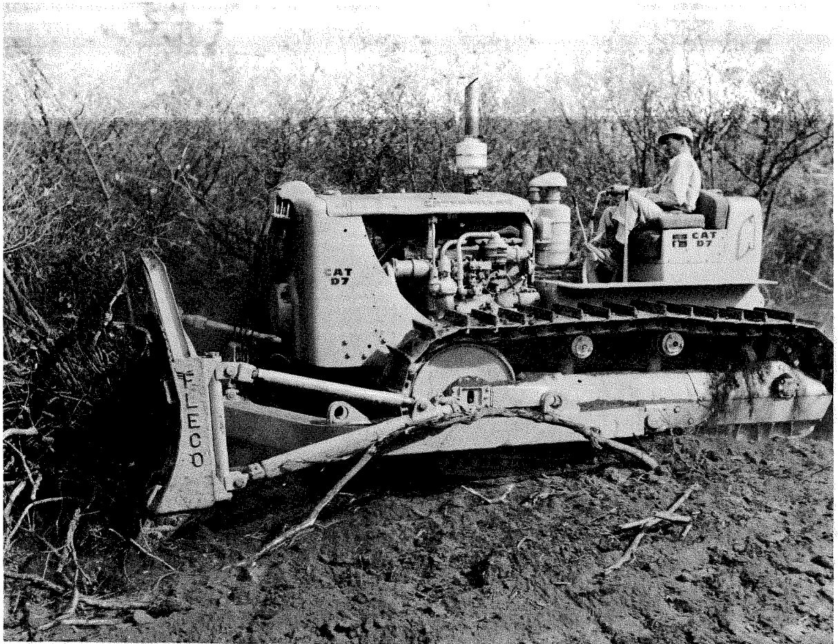
Figure 4. Using a bulldozer with a "root rake" to clear brush from an area to be planted.
