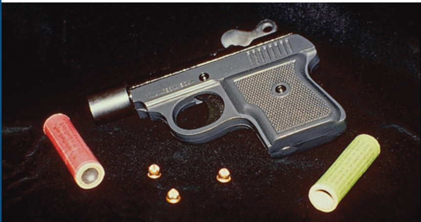
Figure 3. Pistol launcher with bird bomb (left), .22-caliber blanks, and screamer (right). Photo: J. P. Clark, CDFA.
