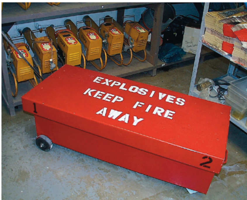
Figure 33. A magazine permits safe storage and legal transport of pyrotechnics. Photo: W. P. Gorenzel.
