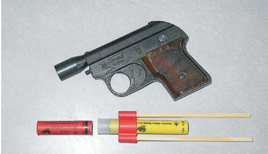
Figure 4. A screamer banger rocket includes a collar to hold the banger over the screamer rocket and wooden stabilizers to control the trajectory. Photo: W. P. Gorenzel.
