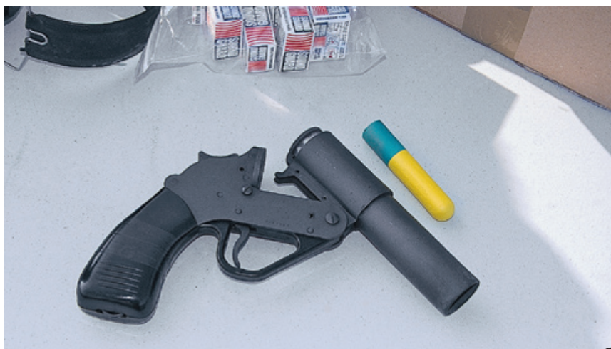
Figure 7. The CAPA launcher, a modified flare gun that fires a small rocket up to 1,000 feet. Photo: W. P. Gorenzel.
