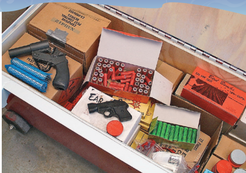
Figure 34. Bird bombs, screamers, shell crackers, CAPA rockets, .22-caliber blanks, and launchers stored in a portable magazine. Photo: W. P. Gorenzel.
