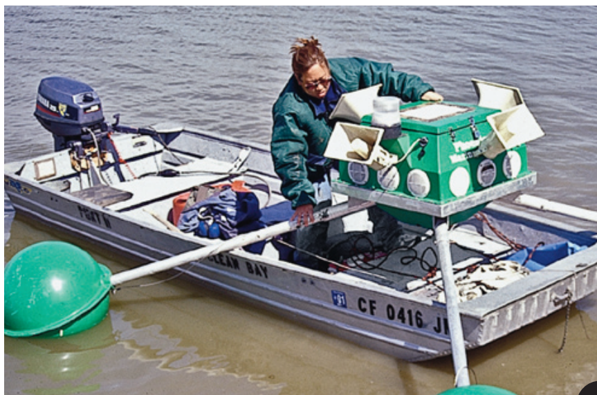
Figure 9. The Marine Phoenix Wailer floats on the water and broadcasts alarm and distress calls. Photo: D. A. Whisson.
