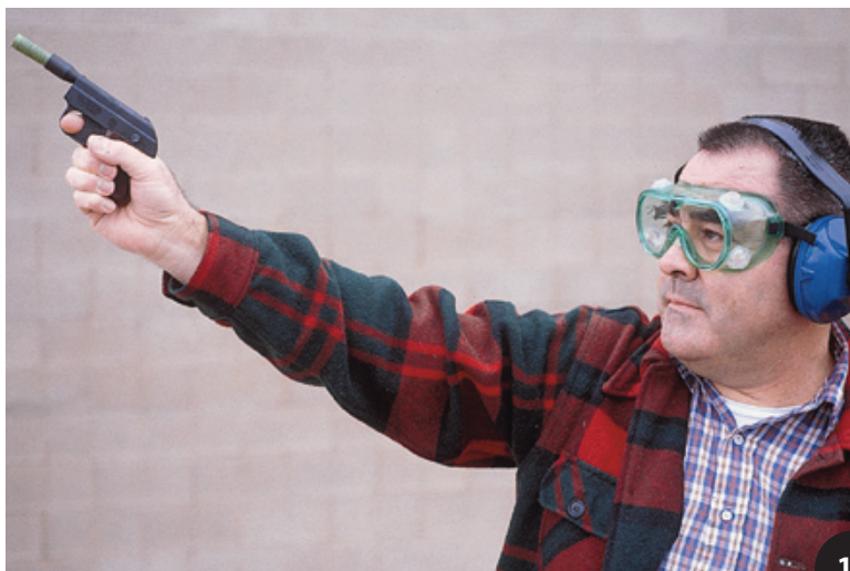
Figure 5. Launcher with bird bomb held at 45° angle. Note eye and ear protection. Photo: J. P. Clark.
