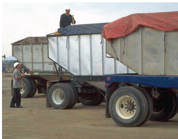
Figure 24. Monitoring temperatures of wild rice curing in bottom-dump trailers.
