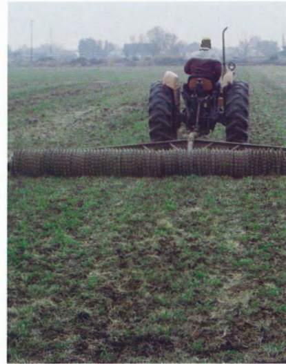
PLATE 7. Rollers are used to firm the seedbed and incorporate seed.
