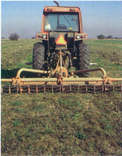
PLATE 5. PTO cultivator preparing a seedbed in tough soil conditions.
