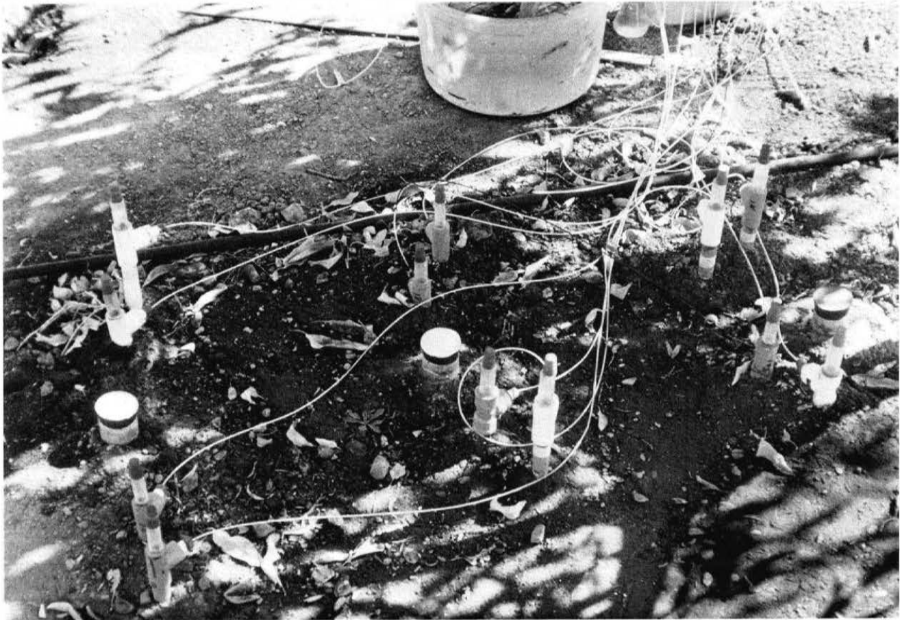
Tensiometers and neutron probe access tubes in place to monitor soil water levels.
