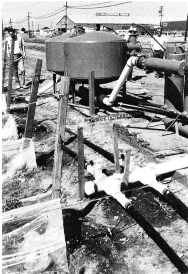
Sand filters being used in drip irrigation of tomatoes.
